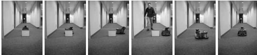
Fig. 3. Individual box-pushing in a corridor. From left to right, a robot perceives the box, reaches and surrounds it. Next the robot pushes the box towards the bar code located at the extreme end of the corridor
