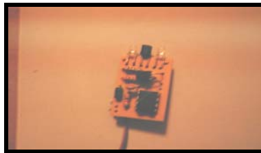
Fig. 1. Binary output sensing device for VR interaction and position detection.
