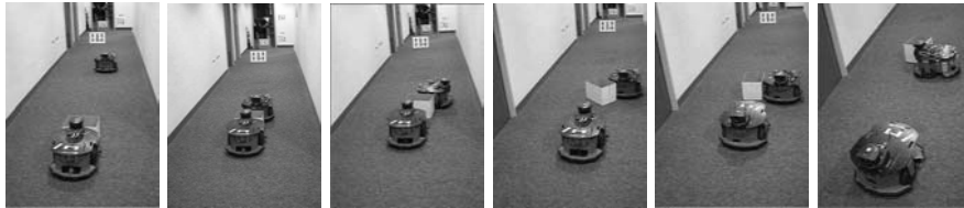
Fig. 5. Sequence of actions executed by robots foraging in a divided corridor. From left to right, robot p03 pushes a box while robot p01 waits in front of its own supplier. p01 tries to reach the box before than p03 finished, producing then a collision
