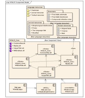
Fig. 4. The components that make up the WS4LR system and their inter-relationships
